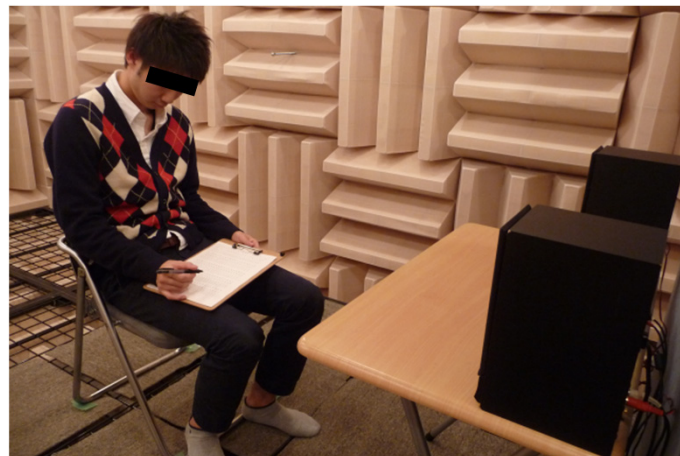
Fig. 3-37 Evaluation setup of whether the rhythmical sounds affect productivity
