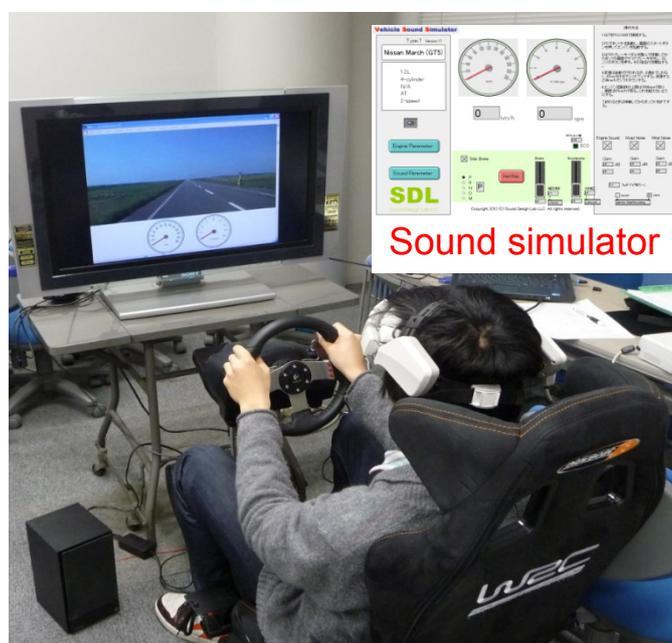
Fig. 4-12 Evaluation setup of sound quality under complex stimuli using driving simulator
