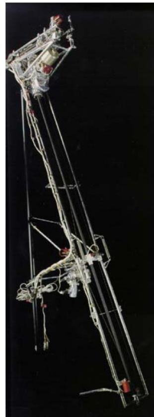
Fig. 1.8 Drilling system during Luna 24 [15]
