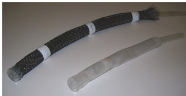
Fig. 6.5 Worm-like robot with discrete actuators surrounded by a braided mesh [84]
