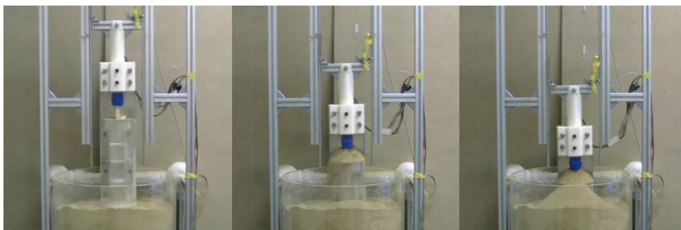
Fig. 5.17 Experimental results of developed excavation unit
