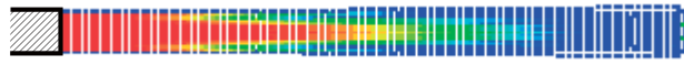
Fig. 3 An example of pressure distribution in a water jet computed by CSP method
