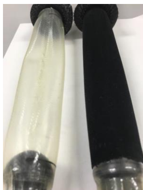
Fig. 1.16 Inner elastomer tube of McKibben pneumatic artificial muscle[42]
