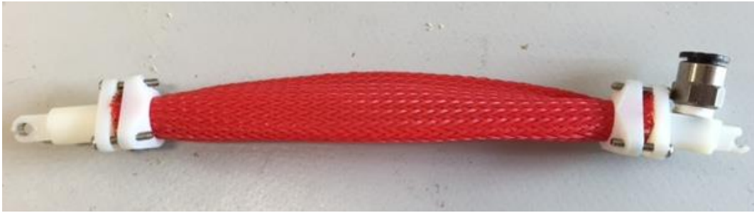
Fig. 1.6 McKibben type artificial muscle
