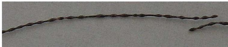
Fig. 5 Melted situation of a copper wire of 0.25 mm in diameter
