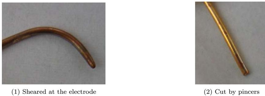
Fig.6 Enlarged broken surfaces of wires (1.0 mm $\Phi$ )
