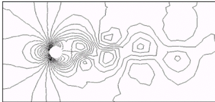
Fig. 4 pressure distribution using conventional analytical model
