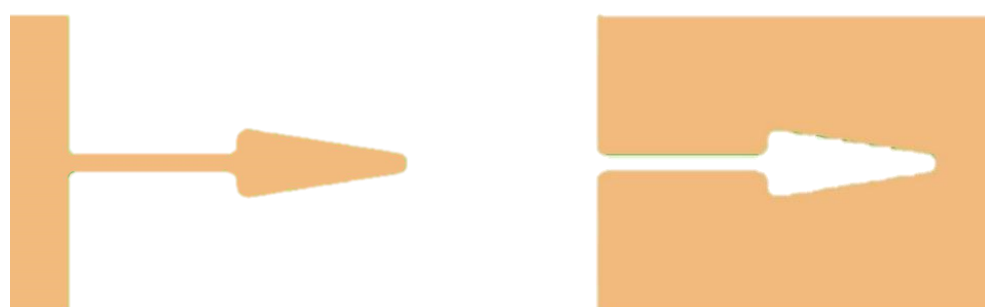
(b) Optimum shape against tensile load (L^*=1.25, D^*=0.0625, S^*=0.2, R^*=0.075)
