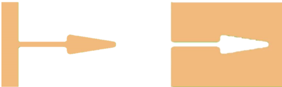
(c) Optimum shape against tensile load (L^*=1.25, D^*=0.0625, S^*=0.2, R^*=0.075)
