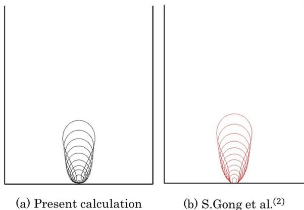
Fig. 7 Bubble growth on a microheater before detachment
