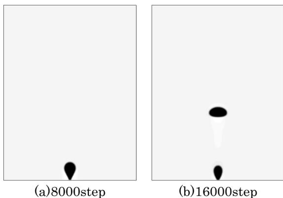
Fig. 8 Computational results of boiling
