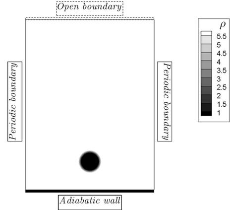
Fig. 4 Computational model of bubble rising
