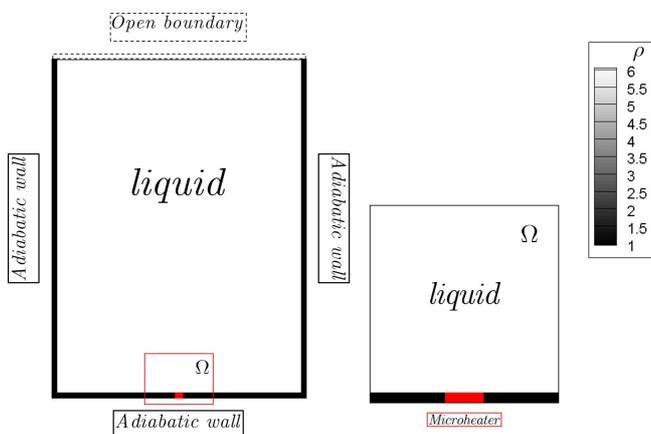
Fig. 6 Computational model of boiling
