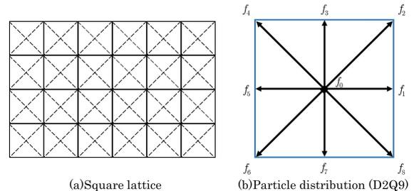
Fig. 3 Particle distribution function
