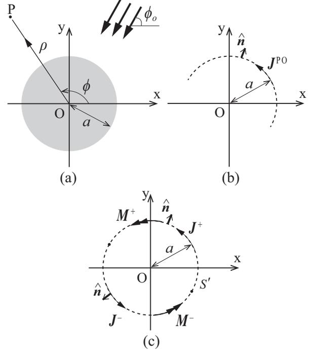
Figure 2: Scattering from a circular conducting cylinder. (a) The circular cylinder illuminated by a plane wave. (b) PO current  $\mathbf{J}^{\text{PO}}$  by the incident field on the illuminated surface. (c) Equivalent currents  $\mathbf{J}^+, \mathbf{J}^-, \mathbf{M}^+, \mathbf{M}^-$  derived by GO fields.
