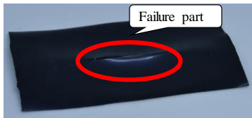
Fig.3 Failure mode of straight-fiber-type artificial muscle.
