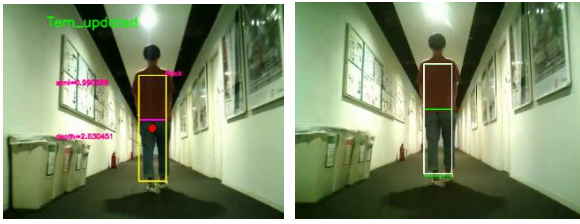
Fig.12 A frame that succeeded in returning to track a person with the proposed method
