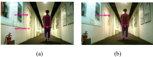
Fig.5 Examples of points used for distance calculation: (a) left camera image (b) right camera image
