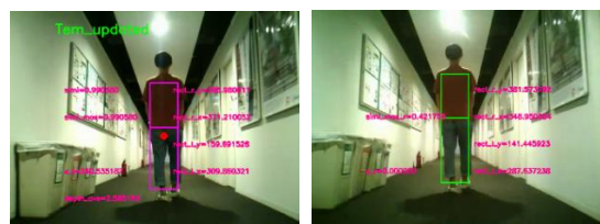
Fig.11 A frame that failed to track a person using the method without a return function
