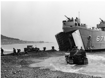
US military Landing Ship, Tank, commonly known as an LST. Source: National Archives of the United States.
