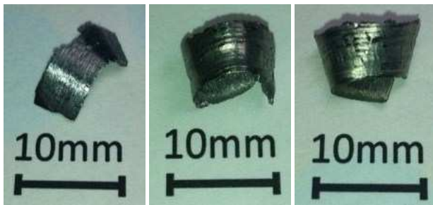
(a) V=10\text{m/min} Thickness=1.37mm (b) V=15\text{m/min} Thickness=1.06mm (c) V=20\text{m/min} Thickness=0.87mm
