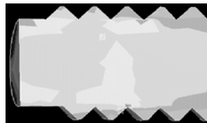
Fig.13 Stress distribution of mating area (3 dimensional FEM)
